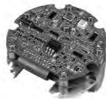
SAU Electronics Assembly for ground to air missile application
