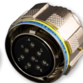
D38999 Series III Shell size 17, 8 channel 40 Grams (less contacts)
