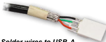
Solder wires to USB-A Insert
