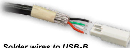
Solder wires to USB-B Insert
