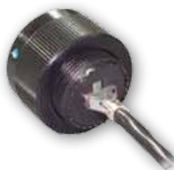
Push terminated USB connector into the dielectric until the tab bottoms in the notch
