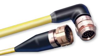
Geo-Marine® plugs are equipped with arctic coupling nuts—made from marine-grade naval bronze with easy-to-grip castellated knurling and a powerful ratcheted anti-decoupling mechanism which quarantees reliable mating and demating performance in even the harshest environments. Supplied as discrete connectors or more typically in build-to-print overmolded cable assemblies.
