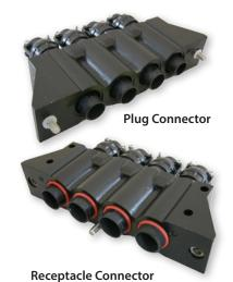
The Glenair IRT series is a rectangular power connector for harsh environmental conditions. Available with three, four and six contacts, typical for traction motor applications. Suitable for single cables AWG 4 – 373MCM (35 to 185 mmq). Working voltage up to 3000 Vcc.
