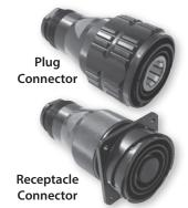
ITS 500 Series derives from an important Military Specification for Power Connectors: VG96929. Suitable for harsh environmental conditions, ITS 500 accepts cable gauges AWG 3/0 to 444MCM (95-240 mmq), for current up to 750 Amp.
