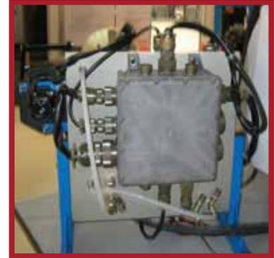
The case was solved with Glenair ITS reverse bayonet connector cables and flange mount receptacles. Plugs with cable clamp backshells mated to receptacles mounted on existing metal junction boxes along with a specially-designed, corrosion-free and EMI/RFI-protected Glenair Composite Junction Box, factory wired to an internal termination block.
