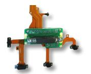
"Best of both worlds" combines durable rigid board areas for doublesided and component mounting with 3-D routing advantages of vibration-resistant flex circuitry
